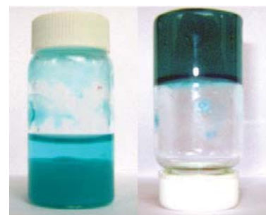
Figure 1. Phase separation (left) or gelation (right) observed upon the complexation of \text{Cu}^{2+} ions with P(Eth-co-MAc) copolymers, depending on the concentration of \text{Cu}^{2+} ions.
