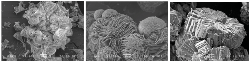
Figure 2: a, b, c are morphologies for 5, 10 and 20% w/w gelatin respectively
